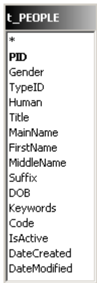
Figure 2-6 Fieldlist A fieldlist is a list showing fields that are in a table or query.
